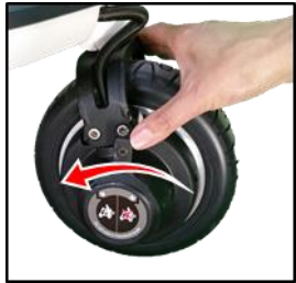
Figuur 52 Securing the freewheel
