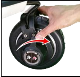
Figuur 51 Releasing the freewheel
